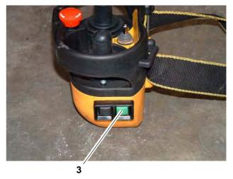
If necessary engine Revs Per Minute (RPM) can be adjusted up (faster) or down (slower) to aid tracking using buttons as shown.
