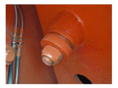
Use a crane with a strap/chain (lifting eye) to lift and hold the wear plate into position. Install and tighten the bolts with the nuts and washers.
