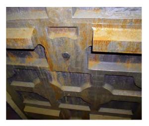
Use the crane and lower the plate into position, SLOWLY into the crusher box. Make sure the a clearance of 10mm to 15mm is between both sides.
