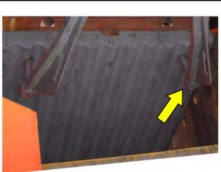
9. Remove the lifting tools and from the swing jaw plate
