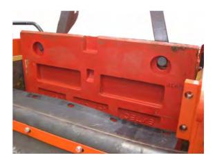
18. When the jaw plate is away from the machine move it down.
