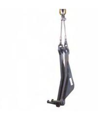
4. Install the Lifting hooks into the lifting eyes correctly. Tighten the chain/ropes with the crane.
