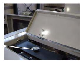
6.10.7. Checking/ Changing Hydraulic Tank Air Breather
