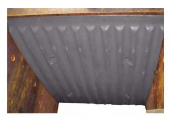
11. Adjust the fixed jaw plate as necessary and make sure it is centred.
