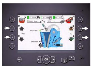
Figure 4-7: Hopper Level Control - Sub Menu
